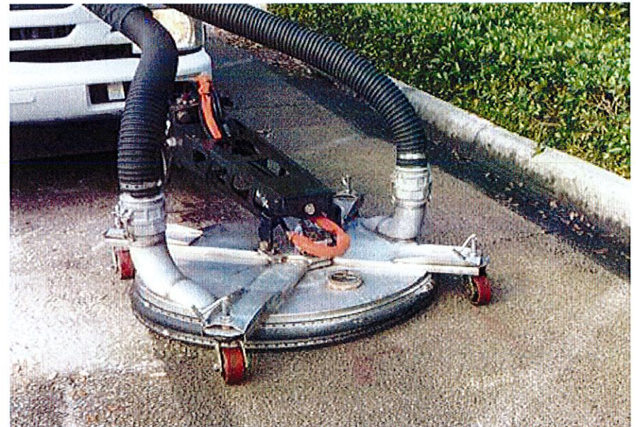
Figure 10: EXAMPLE OF PERVIOUS PAVEMENT VACUUM (Surface Hog)
